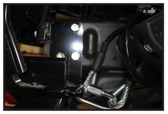
11. Attach the permanent baseplate safety cables to the provided convenience link on the baseplate. The photo above shows the recommended installation of the cables to frame of vehicle. Additional options may interfere with suggested mounting; in this case, secure the cables to a solid piece of the frame as described in the General Information sheet. Be sure the safety cables do not rub against any hoses or moving parts. Do this on **BOTH** sides of the vehicle.
