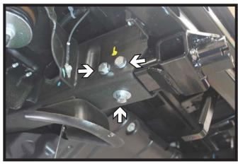
8. Slide the baseplate into the frame pocket and install 1/2"-13 x 1-1/4" bolts with 1/2" lock washers into the outside frame holes and the bottom hole. On the bottom hole use a 1/2" whiz nut on the inside of the frame, using the factory hole for access. Fully tighten all fasteners until the frame squeezes against the baseplate. Do this on both sides of the vehicle.
