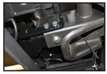
11. Install the convenience link to the frame with 1/2"-13 x 1-3/4" bolts with 1/2" lock washers. Do this on both sides of the vehicle. Tighten down until the frame squeezes against the baseplate.
