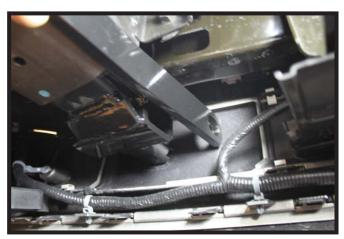
10. Partially reinstall the fascia again. On the inside of the frame, hold the convenience link against the frame and fascia an mark the area to trim. Do this on both sides of the vehicle. Remove the fascia and trim.
