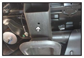
6. Using a 17/32" drill bit, drill out the existing hole in the bottom of the frame. Do this on both sides of the vehicle.
