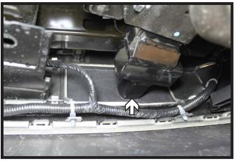
Partially reinstall the fascia with a couple of screws along the top and pull the fascia tight against the baseplate. Trace around the attachment tab tube for trimming (Left). Do this on both sides of the vehicle. Remove and trim out the fascia around the attachment tab tubes.
