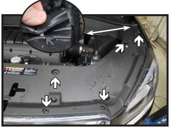
Remove the five (5) push pins from the top fascia cover (white). Then pry up the end of the rubber strip, releasing the clip underneath (gray). Do this on both sides of the vehicle. Remove the cover from the vehicle.
