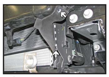
On the driver side, remove the push pin from the top of the plastic air deflector and trim as shown.
