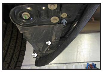
5. Remove two (2) Phillips screws from under the fascia with a screwdriver. Using a 10MM socket, also remove the hex bolt from under the fascia (gray arrow). Do this to both sides. Pull fascia corners to the side of vehicle to release, then pull fascia forward and set fascia aside carefully for later reinstallation along with bolts.
