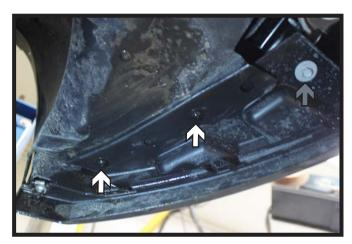
4. On the underside corner of the fascia, using a T20 Torx, remove the two (2) outer screws (white). Then using a 10MM socket, remove the one (1) inner screw (gray). Do this on both sides of the vehicle. Remove the fascia from the vehicle and set aside.
