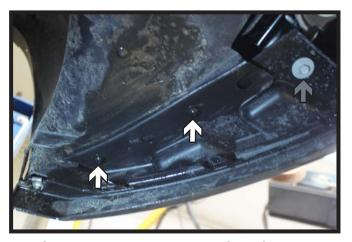
4. On the underside corner of the fascia, using a T20 Torx, remove the two (2) outer screws (white). Then using a 10MM socket, remove the one (1) inner screw (gray). Do this on both sides of the vehicle. Pull the corners of the fascia away from the vehicle disconnecting any electrical connections and set the fascia aside.
