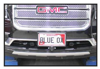
9. Hold the fascia as close to its original position, mark and trim the fascia around the convenience links and attachment tabs. Reinstall the fascia and fascia cover.
