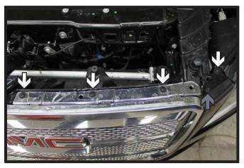
Along the top edge of the fascia, using a T20 Torx, remove the four (4) screws from the driver side (white). Then the three (3) on the passenger side. Using a 7MM socket, remove the screw from the edge on both sides of the vehicle (gray).
