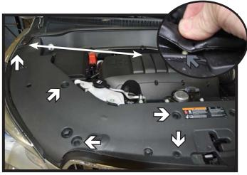
Remove the five (5) push pins from the top fascia cover (white). Then pry up the end of the rubber strip, releasing the clip underneath (gray). Do this on both sides of the vehicle. Remove the cover from the vehicle.
