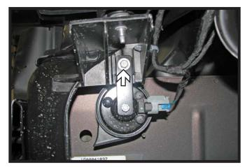
7. Using a 10MM socket, remove the screw from the horn bracket and set horn aside. Do this on both sides of the vehicle.
