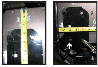
9. Tip the baseplate onto the frame. Measure down 2-13/16" from the top of the frame to the top of the baseplate. Measure 6-1/4" from the front of the frame to the back of the baseplate. Level the baseplate and clamp into position. Using the baseplate as a template, drill a 13/32" hole (white) and insert a 3/8"-16 x 1" hex bolt, 3/8" lock washer and 3/8"-16 hex nut. Do this to both sides of the vehicle. Tighten down fasteners.
