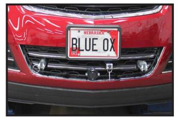
15. Hold the fascia as close to its original postion, mark and trim the fascia around the convienence links and attachment tabs. Reinstall the fascia and fascia shroud.
