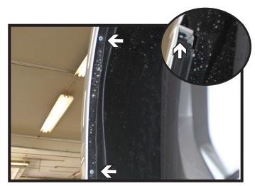
3. **2013 Models:** Using a T20 Torx, remove the three (3) screws from the outer edge of the wheel well. Do this on both sides of the vehicle.
