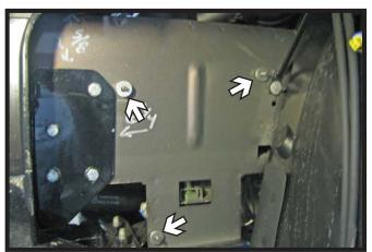
On the driver side, place six (6) 1/4" flat washers onto each of the washer reservoir studs. Reinstall the reservoir and horns.
