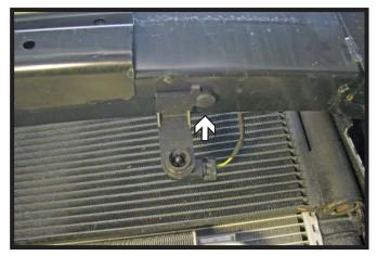
6. On the driver side, remove the push pin from the temperature sensor and temporarily move above the bumper. The sensor will be relocated later.
