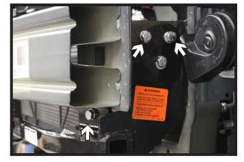
14. Drill the remaining two (2) holes at the top of the endplates and the front hole thru the frame. Install the 3/8" hardware and fully tighten all fasteners. Do this on **BOTH** sides of the vehicle.
