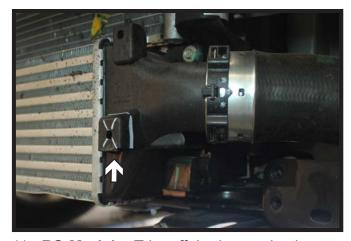
11. **RS-Models:** Trim off the lower plastic shrouding mount as shown above for baseplate clearance. Do this on both sides of the vehicle.
