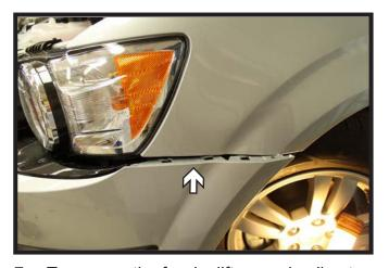
7. To remove the fascia, lift up and pull out at the fascia seam by the wheel wells. Disconnect any electrical connections and remove the fascia.
