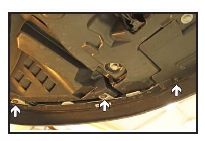
3. Using a T20 Torx, remove the six (6) screws from the underside of the fascia. There are three (3) on each side.
