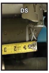
12. With a reciprocating saw, notch over 1" from the edge and upward to just slightly under the bumper. Do this on **BOTH** sides of the vehicle.
