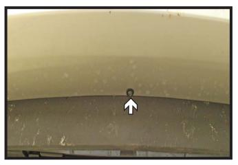
5. Underneath the license plate, with T20 Torx, remove the one (1) screw. Remove the front portion of the belly pan.
