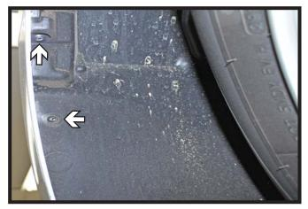
2. In the wheel well, using T20 Torx, remove the four (4) screws. Do this to both sides of the vehicle.
