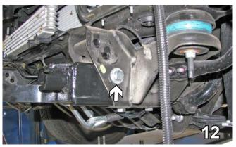
12. Insert 1/2-13 x 1 1/4" hex bolts with 1/2" lock washers into both sides of the base plate. Be sure to use Loctite red on all bolts. Do this on both sides of the vehicle.
