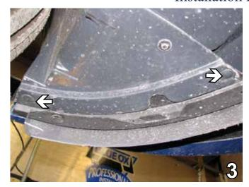
Just forward of the front tires, on the under side of the front fascia, remove two push pins. This is done on both sides of the vehicle, the driver's side is shown. Set the push pins aside to be reinstalled later. Pull fascia forward and set aside carefully to be reinstalled later.
