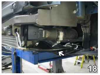
18. Attach permanent baseplate safety cables to the quick link on the baseplate. On the driver's side, the cables go straight back and around the frame of vehicle. Additional options may interfere with suggested mounting, in this case secure the cables to a solid piece of the frame as described in instructions included with the permanent baseplate safety cables. Be sure the safety cables do not rub against any hoses or moving parts.
