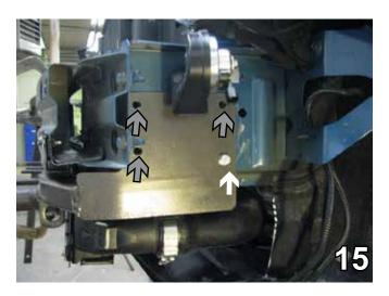
15. Insert a 3/8-16 x 1 1/4" hex bolt with 3/8" lock washer into the existing hole (white arrow). Be sure to use Loctite. Attach it to a 3/8-16 nut plate. Using the baseplate as a template, drill the three remaining holes (gray arrows) with a 13/32" drill bit. This is done on both sides of the vehicle.
