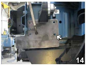
14. Align the baseplate with the existing hole. Clamp across the top of the frame with the large vise grip. This is done on both sides of the vehicle.
