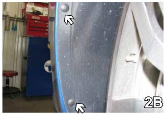
Just forward of the front tire, remove one 7MM bolt with the 7MM socket (see grey arrow) and remove two push pins (see white arrows). This is done on both sides of the vehicle, the driver's side is shown. Set all aside to be reinstalled later.
