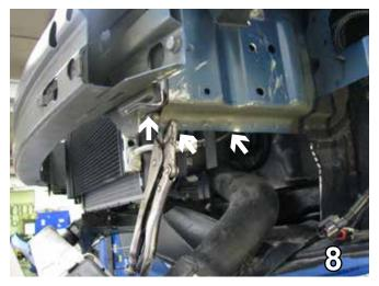
8. Using a vise grip, bend up where we just cut and continue to bend back to the middle of the rib. This is done on both sides of the vehicle.
