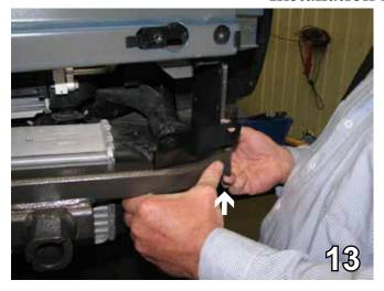
Continue to move the baseplate and the turbo on up into position. This is done on both sides of the vehicle.
