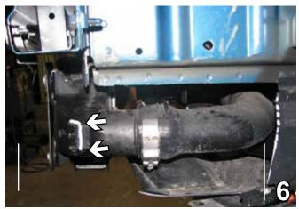
6. Trim the notch off the end of the tube but be careful not to touch anything else. This is done on both sides of the vehicle, the driver's side is shown,
