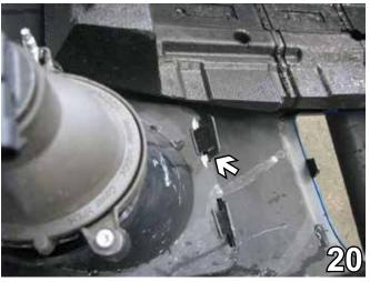
20. On the back side of the fascia, use a utility knife to cut the tall tab off. This is done on both sides of the vehicle. Reinstall the front fascia.
