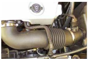
**5.** Loosen the two hose clamps from engine air intake and filter assembly, slide hose ends off, disconnect small tube from lower side of intake end and set aside.
