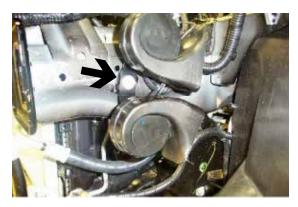
8. Remove metric bolt from horn bracket on driver's side, unplug the electrical connection and set aside.
