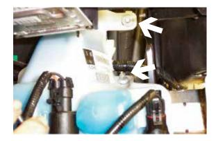
**9.** Just above washer reservoir on driver's side are two metric bolts to remove with the 10MM socket.
