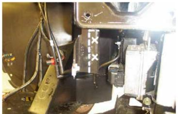
**16.** Locate front washer reservoir bracket on the passenger's side, measure 1/2" from bracket edge and up to bumper bracket, remove this portion of bracket with the reciprocating saw This will prepare area for baseplate installation.
