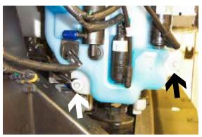
**10.** Remove metric bolt from lower washer reservoir and front bracket with the 10MM socket.
