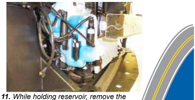
While holding reservoir, remove the metric bolt between wheel well and reservoir with the 10MM socket. Unplug electrical lines, disconnect and plug fluid lines, set reservoir aside.
