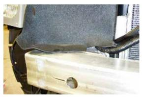
**14.** Remove four push pins from air dams on metal bumper.
