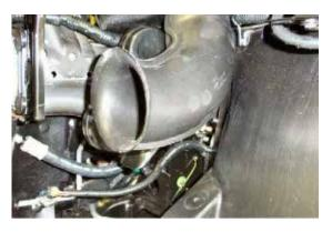
7. Using the 10MM socket, remove two metric bolt from filter assembly, lift assembly tube end out of fender and engine compartment, set aside.
