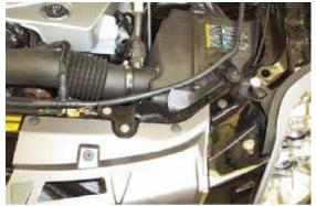
**1.** Remove the four push pins from top edge of fascia, both sides.
