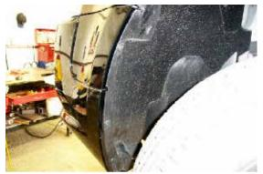
**2.** Just forward of front tire on edge of wheel well are three push pins to remove, both sides.
