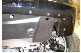
**4.** Remove 12 push pins from lower edge of fascia, pull fascia forward, disconnect electrical plug from light assembly and set fascia aside.
