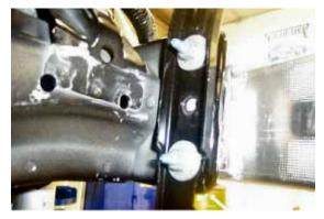
**15.** Using the 10MM deep well socket, remove the four metric bolts from the back side of bumper bracket, both sides and pull metal bumper forward, set aside.
