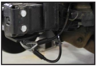
13. Attach the permanent baseplate safety cables to the provided convenience link on the baseplate. The photo above shows the recommended installation of the cables to frame of vehicle. Additional options may interfere with suggested mounting; in this case, secure the cables to a solid piece of the frame as described in the General Information sheet. Be sure the safety cables do not rub against any hoses or moving parts. Do this on **BOTH** sides of the vehicle.
