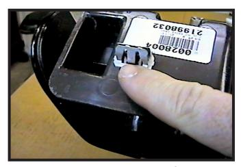
4. Remove all seven metal clips from the metal frame and reinstall them to the tabs on the back side of the grille.
