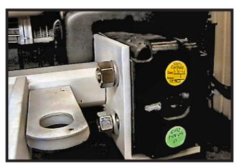
12. Remove the four (4) hex nuts from the 1/2" x 3-1/2" bolts. Install lock washers and fully tighten all fasteners.
