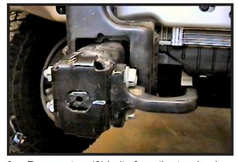
8. Remove two (2) bolts from the tow hook using the 18MM socket. Do this to both sides of the vehicle.
