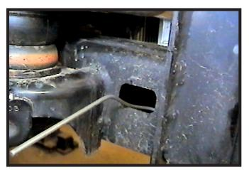
11. Insert a nut plate into the opening just behind the drilled hole on the outside of the frame to align with the drilled hole. Install a 1/2"-13 x 1-3/4" bolt with lock washer into the bottom hole.
