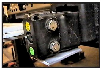
9. Hold up the baseplate up and align with the existing tow hook holes. Insert 1/2"-13 x 3-1/2" bolts into the holes. Be sure that baseplate is level with the vehicle and temporarily tighten with a nut.
