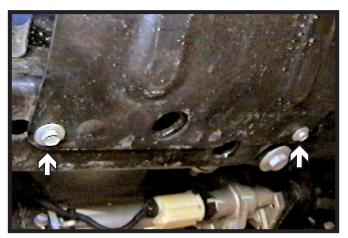
5. Remove the four (4) bolts from the belly pan using the 13MM socket, pull the belly pan down to remove. Set the belly pan aside.
