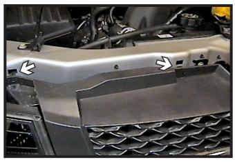
1. Push down on the four (4) retainer clips to release the grille.
