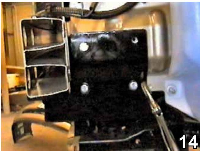
14. Insert the nutplate into the opening on the bottom of the frame (see photo 13) to align with the upper drilled hole on the driver's side, tighten the lock washer and hex nut.
