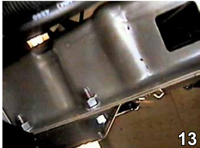
13. Insert two 3/8" bolts into the lower holes in the baseplate. Tighten the lock washer and the hex nut. Do this to both sides of the vehicle.
