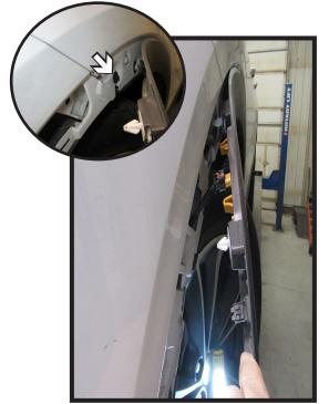
Pull back the wheel well trim and prop away from the vehicle using a soft cloth. Then using a 7MM socket remove the one (1) bolt from the fascia joint (inset). Do this on both sides of the vehicle.
