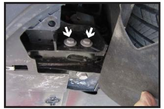
6. Gently pull back lower cover. Using a 13MM socket, remove the two (2) bolts from the underside of the facia. Do this on both sides of the vehicle. Remove fascia and set aside to be reinstalled later.
