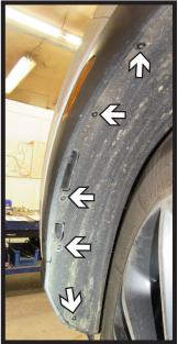
2. Using a T15 Torx, remove the five (5) bolts from along the edge of the wheel well. Do this on both sides of the vehicle.
