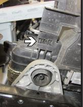
8. Remove the shroud below the bumper by cutting the indicated area (left). Then press clip on bottom of shroud to slide forward and off of the vehicle (right). Do this on both sides of the vehicle.
