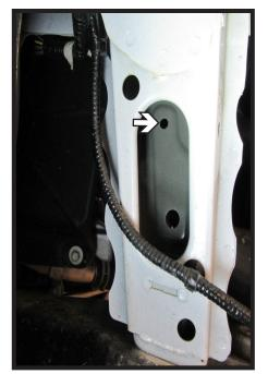
10. Using a 1/2" drill bit, drill out the top hole on the passenger side of the vehicle.
