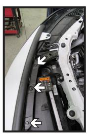
Using a T15 Torx, remove the six (6) bolts from the top edge of the fascia. There are three (3) on the passenger side and three (3) on the driver side of the vehicle.
