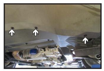
5. Using a 7MM socket, remove the ten (10) screws from the underside of the fascia. There are five (5) on each side.
