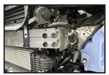
Using a reciprocating saw, trim the end of the bumper flush with the outside of the frame. Do this on both sides of the vehicle.
