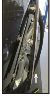
4. Pull back the wheel well liner. Using a 10MM socket remove the bolt (gray arrow). Then release the clips from the fender flare (left, white arrow). Pull straight up on the flare to release the bottom and then out away from the vehicle. Do this on both sides of the vehicle.
