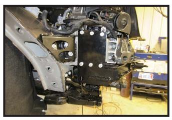
11. Flush the baseplate with the top and front lips of the frame (gray). Level and clamp into position.
