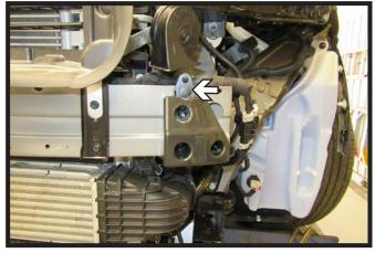
9. Remove the push pin from plastic reinforcement on the bumper face and set aside. Do this on both sides of the vehicle.
