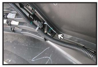
14. On the backside of the fascia, trim the lower tab back flush with the lip. Do this on both sides of the fascia.
