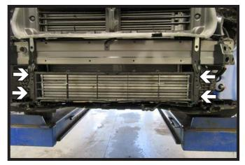
Using a 25 Torx socket, remove the four
