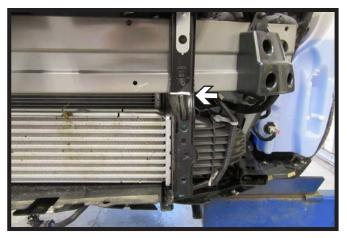
7. Using a reciprocating saw, trim the bracket flush with the bottom side of the bumper. Do this on both sides of the vehicle.
