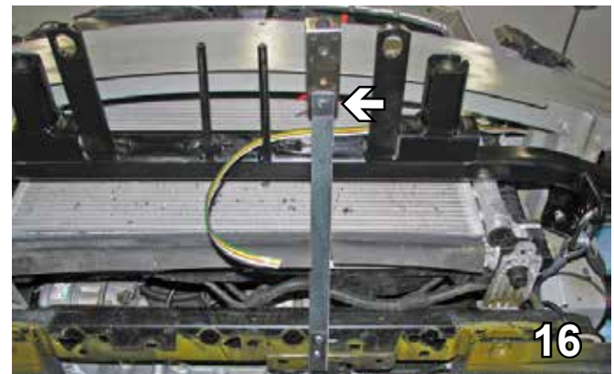
15. Attach the breakaway bracket to the frame cross member with two 10-16 x 1" self drilling screws.
