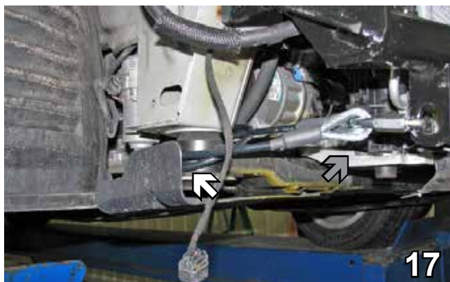
16. Attach the breakaway to the bracket with 1/4-20 x 3/4" hex bolt and 1/4-20 hex nut.
