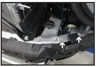
On the driver side, using a T30 Torx, remove the two (2) screws from the horn bracket. Disconnect all lines and set the horn assembly aside.
