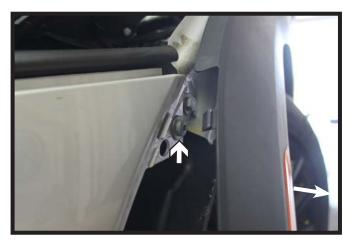
Pry the fender flare away from vehicle. Using a T30 Torx, remove the screw from behind the fender flare. Do this on both sides of the vehicle.
