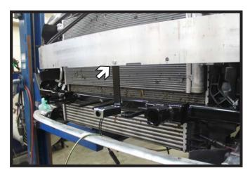
16. **Optional:** Attach the breakaway bracket to the bumper in the desired location with the supplied 1/4" hardware.
