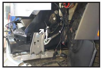
17. On the driver side, ziptie the temperature sensor securely.
