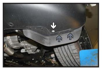
Using a T25 Torx, remove the screw from the underside of the fascia (white). Then the two (2) push pins next to the screw (gray). Do this on both sides of the vehicle.
