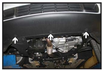
8. Remove the three (3) push pins from the underside of the fascia towards the middle of the vehicle.
