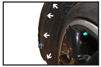
5. Using a 8MM socket, remove the screw from edge of the wheel well (gray). Then remove the four (4) push pins along the edge. Do this on both sides of the vehicle.
