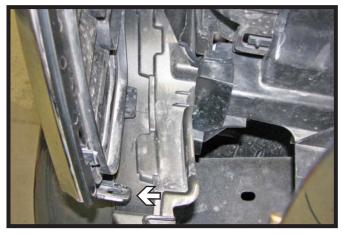
2. Reach down underneath the corner of the headlight, push down on the clip on the corner of the grille and pull to release. Do this on both sides of the vehicle.
