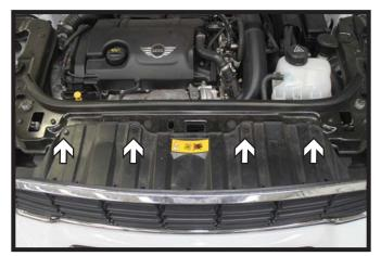
Using a 10MM socket, remove the four (4) screws from the fascia cover and set aside.
