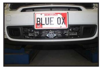
24. Hold the fascia as close to its original position, mark and trim the fascia around the convenience links and attachment tabs. Reinstall the fascia, grille and fascia cover.
