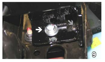
Trim the threads off the outer bolt flush with the nut (gray). Do this on both sides of the vehicle.
