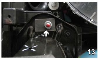
13. On top of bumper, remove nut and replace with 1" x 1.5" nut with Loctite applied. The hole is located 1" in, and you will need one for both sides.
