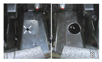
Using an existing hole on top of the metal bumper drill a hole using a 1 1/4" hole saw to cut opening for front end to install nut plates. Do this on both sides.
