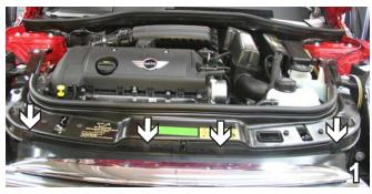
Using a flat screwdriver, remove four pushpins on top edge of grille. Set push pins aside to be reinstalled later.
