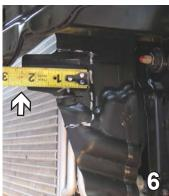
6. You will need to cut the air dams 3" down and 2.5" in to make room for the baseplate. Do this to both sides. These will not be reinstalled.
