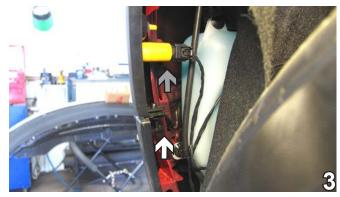
After removing the wheel well cover, remove one pushpin connecting the fascia using a flat screwdriver. Also remove the small yellow light (gray arrow). Do this to both sides. Set pushpins aside for later reinstallation.
