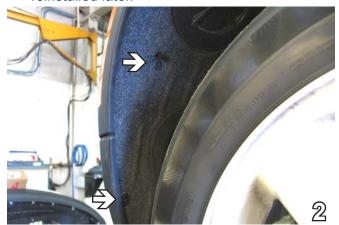
2. Forward the front tire, there are two pushpins that need to be removed. Do this to both sides. Use a flat screwdriver and set aside for later reinstallation.
