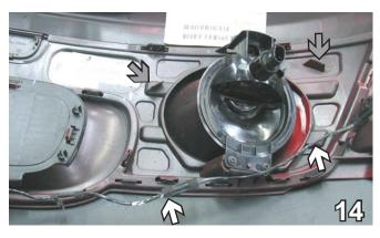
14. The wire air sensor needs to be moved behind the fog light. It originally was placed around the top of the fog light (gray arrows) and needs to be placed and taped below the fog light. Cut off a clip and tape to the sensor below the fog light.
