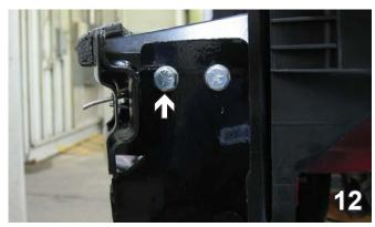
12. Into the holes drilled in the side also insert 3/8-16 x 1 1/4" bolts with Loctite, 3/8" lock washers and 3/8" nut plates. Do this on both sides.
