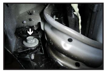
Pull back the wheel well liner. Using a 10MM socket, remove the one (1) bolt from the fascia joint. Do this on both sides of the vehicle.
