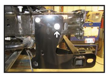
5. Remove the top front bolt and insert frame bracket between the frame and the baseplate. Make sure the bracket is flush with the front of the frame. Reinstall bolt and hardware. Do this on both sides of the vehicle.
