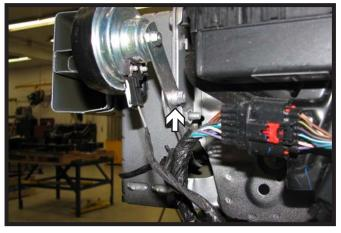
6. Using a 10MM socket, remove the screw from the horn bracket and set the horn aside.
