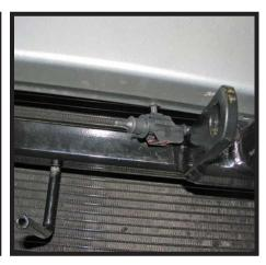
17. Using the 1/4" drill bit, drill a hole in the bottom of the bumper to the inside of the attachment tab (left). Thread the temperature sensor thru the end of the bumper and out the backside (middle). Attach the sensor underneath between the bumper and the baseplate where the hole was drilled (right).
