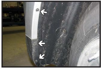
2. Using a 7MM socket, remove the three (3) screws from along the edge of the wheel well. Do this on both sides of the vehicle.
