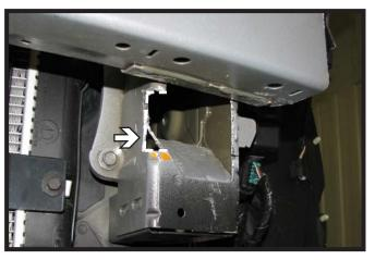
10. On the inside of the frame, make a 2" long notch just under the bumper back about a 1/2" for baseplate clearance. Do this on both sides of the vehicle.
