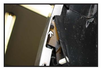
Pull back the wheel well liner, then using a 7MM socket, remove the screw from the fascia/fender joint. Do this on both sides of the vehicle.
