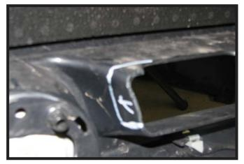
Hold the fascia up to the vehicle and trim the plastic intake slots as needed to clear the baseplate.
