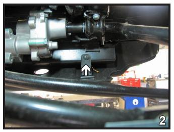
Using a Phillips screwdriver, remove the two (2) push pins from tabs on the backside of the belly pan. Set the belly pan aside.
