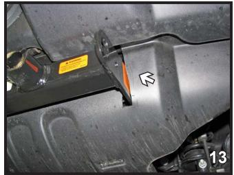
13. Hold the belly pan up to its original position, mark and trim a slot for baseplate endplate to come through with the utility knife. Do this to both sides of the vehicle. Slide the belly pan between baseplate crosstube and lower frame suspension. Allow endplate to come through slot and reinstall the belly pan to its original location.
