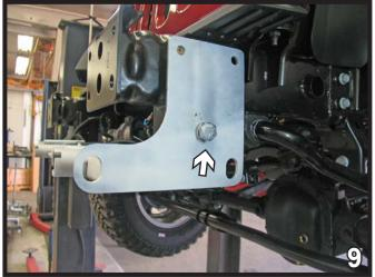
Insert the 5/8"-11 whiz nut into the frame end and align with the lower hole on the 2007-09s and the middle hole on the 2010s and newer. Install the 5/8"-11 x 1-1/2" hex bolt and 5/8" lock washer and tighten to whiz nut. Do this on both sides of the vehicle.
