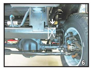
6. **On the 2007-09 models:** Using the reciprocating saw, cut the lower frame extension flush with the outside edge of the lower side bracket. Do this to both sides of the vehicle. We recommend painting the cut edges to prevent them from rusting.
