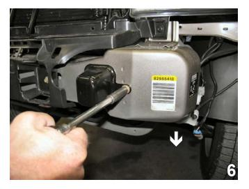
6. Using the 10MM socket to remove one (1) metric bolt. Do this to both sides of the vehicle. Set metric bolts aside to be reinstalled later. Remove the tow hook assembly with the 12MM socket. The tow hooks will **NOT** be reinstalled.
