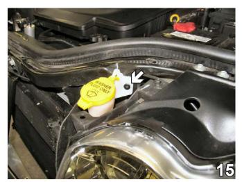
15. Tighten the 1/4"-20 x 3/4" bolt and flat washer into the existing bolt hole of upper reservoir spout. Tighten the 1/4" lock washer and hex nut on to the back side of the radiator support.
