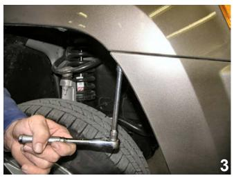
Using a 7MM socket, remove one (1) metric bolt from just forward of the front tire, on the fascia's corner. Do this to both sides of the vehicle. Set the bolts aside to be reinstalled later.
