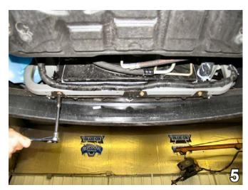
5. Using the 10MM socket, remove three (3) metric bolts from the lower radiator cross member. Pull the fascia forward, unplug the electrical connections. Set the fascia and the bolts aside carefully to be reinstalled later.
