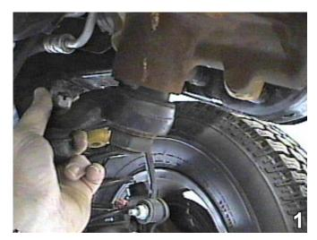
Remove three (3) metric bolts with the 16MM socket while having someone hold the gear box and the idler arm. Set metric bolts aside to be reinstalled later. Do this to both sides of the vehicle.
