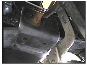
Clamp the passenger's side with the large vise grips. Using the baseplate as a template, drill four (4) holes using the 13/32" drill bit.
