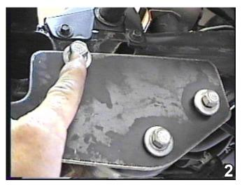
Hold the baseplate into place and insert the three (3) existing bolts on the driver's side through the baseplate, frame, gear box, and tighten.
