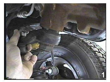
1. Using a 16MM socket, remove three (3) metric bolts, while having someone hold the gear box and the idler arm. Set the bolts aside to be reinstalled later.
