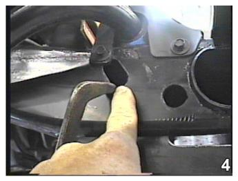
4. Using the 3/8"-16 x 1-1/2" hex bolts, 3/8" lock washers, and the 3/8"-16 nut plates, insert the nutplate into the frame and align with the holes. Tighten ALL bolts.
