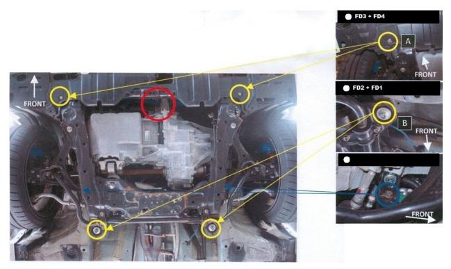
4. Please match the imprinted part numbers on each collar to the appropriate position and orientation shown in the diagram.
