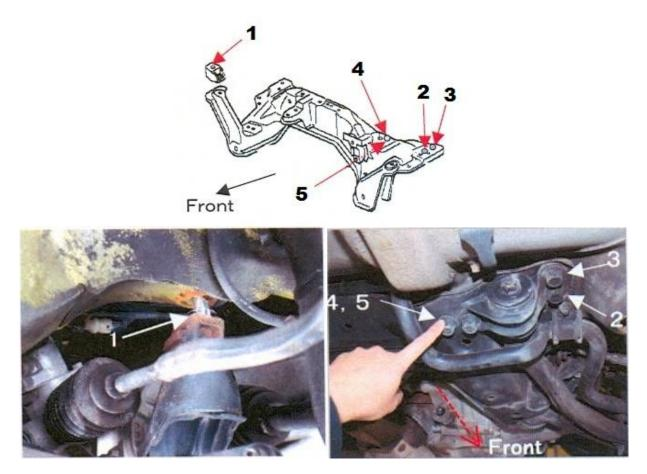
4. Please match the imprinted part numbers on each collar to the appropriate position and orientation shown in the diagram.
