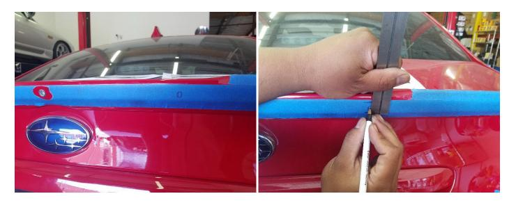
Step 9: While the Gurney Flap is temporarily mounted at the center, trace the remaining holes with a pencil or pen. The remaining hole-centers will be measured using the same methods and steps just completed in locating the center hole.
