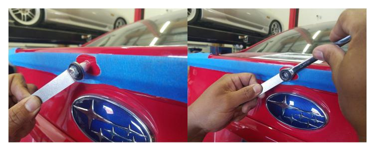
Step 8: Test fit and align the BLOX Racing Gurney Flap using the center hole and hardware you just removed. This will help you mark the remaining holes.
