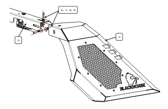
Step 3: Connect brackets and roll bar with standard parts 1 1 1 1 1 1 2 2 as figure shows.
