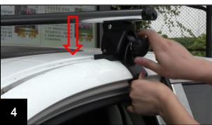
Step 3: Inspect the cross bar if it is in correct position, if yes, make sure to tighten all the bolts. If not, adjust the bolts to the right position, then tighten.
