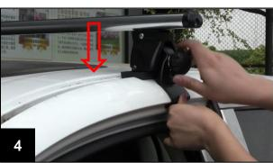
Step 3: Inspect the cross bar if it is in correct position, if yes, make sure to tighten all the bolts. If not, adjust the bolts to the right position, then tighten.
