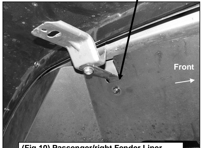
(Fig 10) Passenger/right Fender Liner attached to Top Rear "L" Support Bracket
