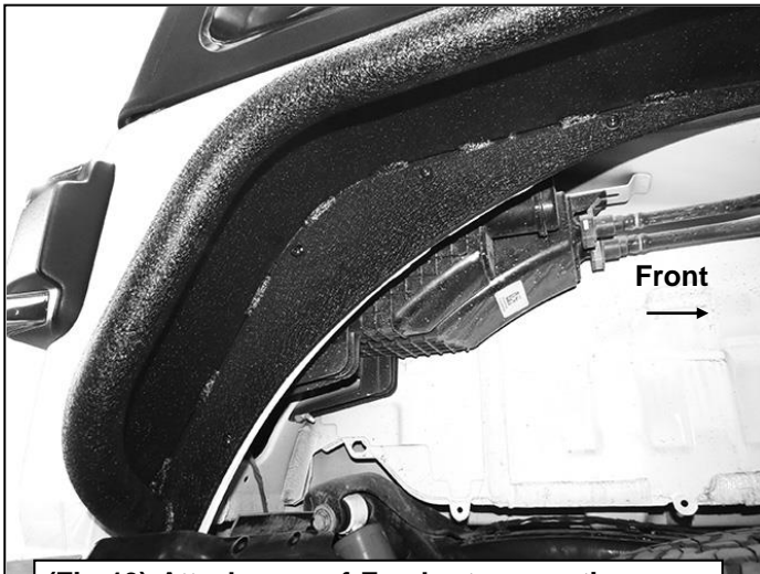
(Fig 13) Attach rear of Fender to mounting locations on body, (passenger/right Fender)
