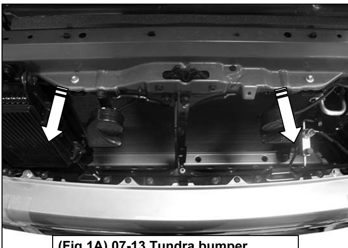
(Fig 1A) 07-13 Tundra bumper bracket location pictured from above
