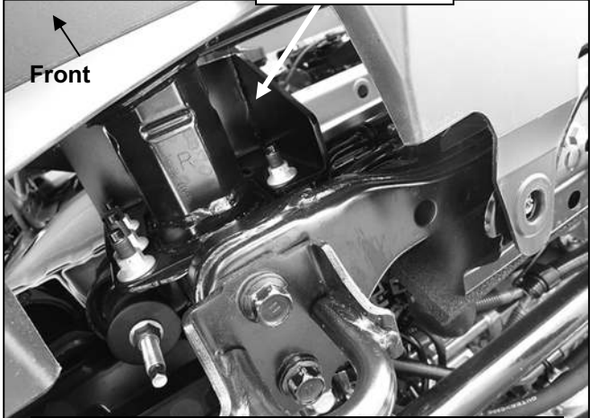
(Fig 4) Reuse factory hex nuts to secure Top Bracket to end of frame. Remove tow hooks
