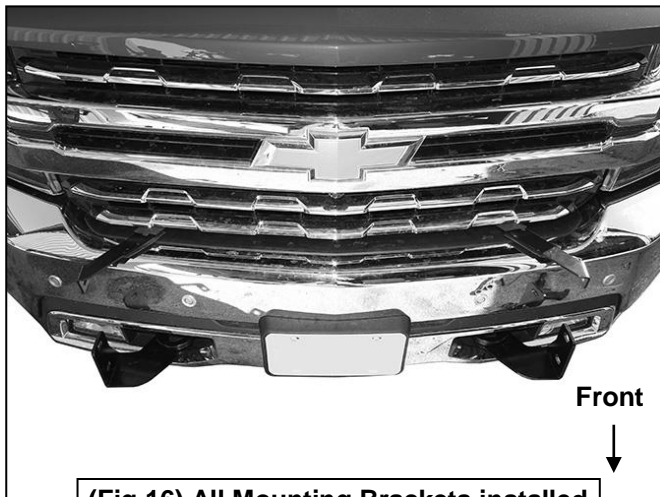
(Fig 16) All Mounting Brackets installed
