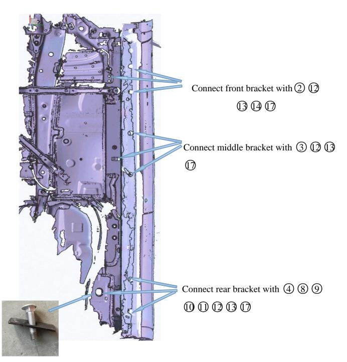
(The way to install T-shaped bolt combo: install the square plate into the square neck bolt, then screwing in the spring. Screwing down the spring after inserted the T-shaped combo into the chassis hole.)
