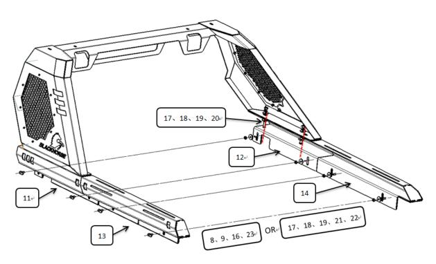
Step 4: Test and make sure that the roll bar is steadily fixed, fully tighten all hardware.
