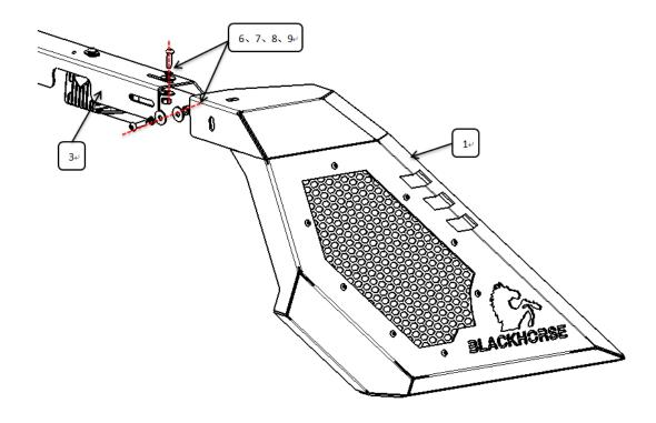
Step 3: Connect brackets and roll bar with standard parts 1 1 1 1 1 2 as figure shows.
