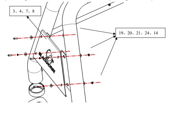
S/S UNIVERSAL ROLL BAR FOR 1/2 TON TRUCKS (GM SILVERADO 2015-FORD F150 2015) FLAT BASE WITH LED BRAKE LIGHT Step 4: Using wrench 13, install support plate 10 and gum cover 9 with part 26.
