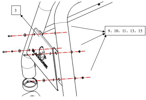
Step4: Using wrench 7, install support plate 6 and gum cover 8 with part 12.
