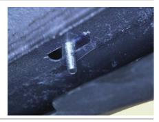
Place an L-shaped hanger bracket onto the vehicle and secure with an M8 flat washer, M8 lock washer and M8 hex nut.
