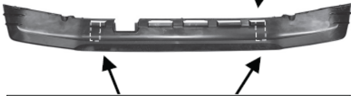
(Fig 10) Dashed lines represent approximate area to cut from air dam and are illustrated for example only
