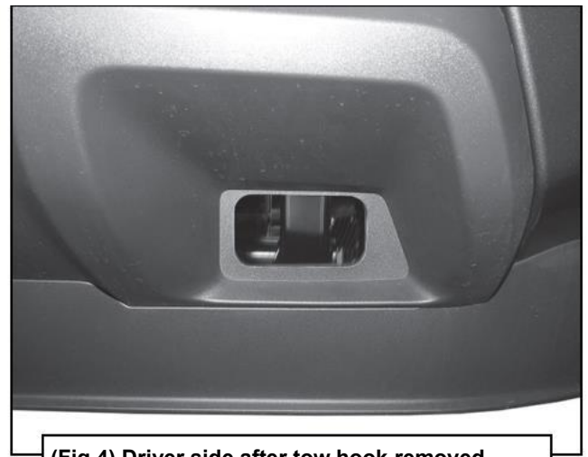
(Fig 4) Driver side after tow hook removed
