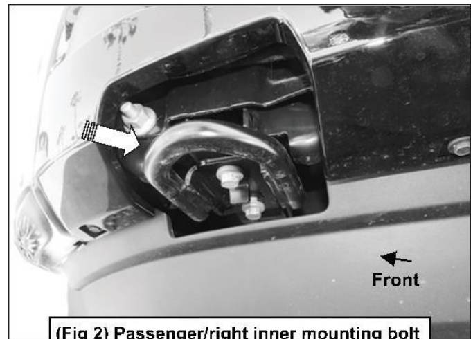
(Fig 2) Passenger/right inner mounting bolt for tow hook pictured from behind bumper
