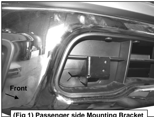
(Fig 1) Passenger side Mounting Bracket inserted through cover
