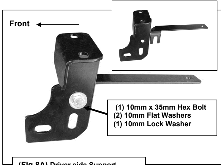
(Fig 8A) Driver side Support Bracket in "no Tow Hook" position
