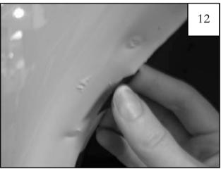
Install Tab (MT1-0014) on sheet metal centered over mark.
