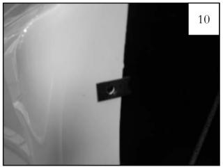
Install Clip (CL1-0011) over existing factory hole.
