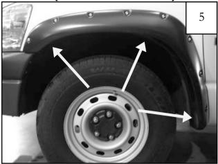
Hold flare to vehicle and reinstall three factory screws with 8mm socket wrench.
