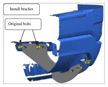
Step 3: Install the bracket-A on the bracket-B by part (6789), Do not tighten all of them.
