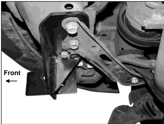
(Fig 3) Passenger/right Mounting Bracket installed
