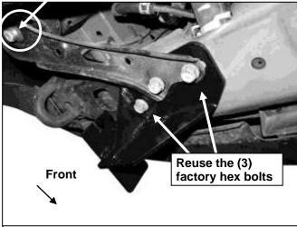
(Fig 2) Driver/left side Mounting Bracket installed
