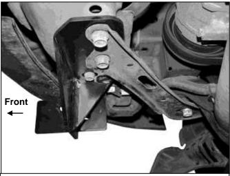
(Fig 3) Passenger/right Mounting Bracket installed
