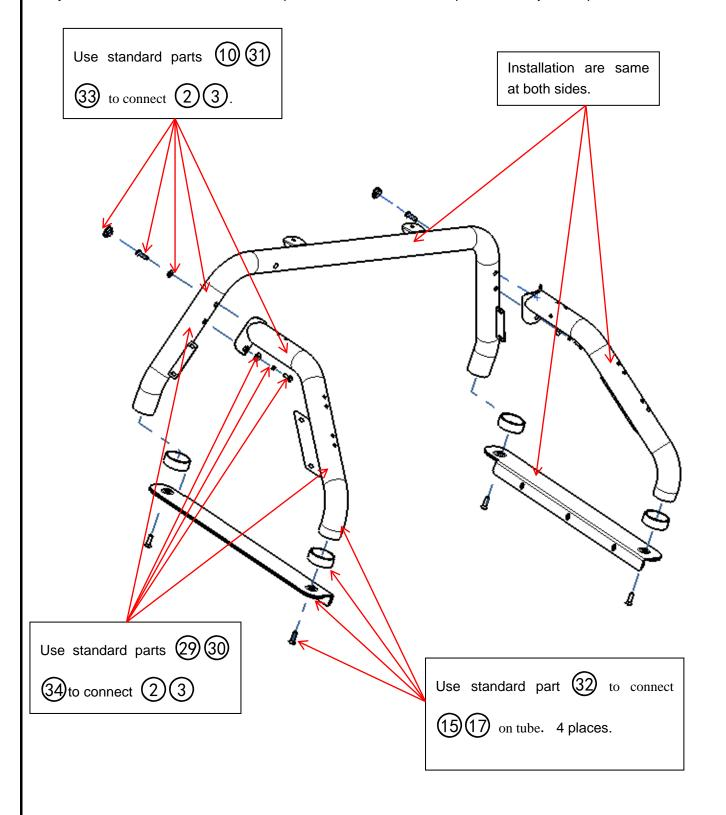
**Step2:** Assemble Luggage frame and tubes with standard parts. Lock all the standard parts after adjust the position.
