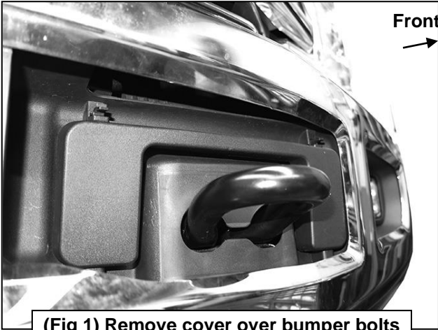
(Fig 1) Remove cover over bumper bolts
