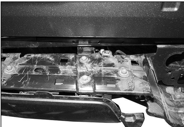
(Fig 3) Models with receiver hitch, remove the hex bolts attaching bumper to top of hitch
