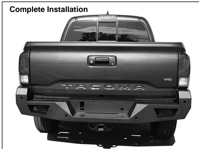
(Fig 13) Model with factory receiver hitch: Attach Bumper to side and bottom of hitch (driver/left installation pictured)
